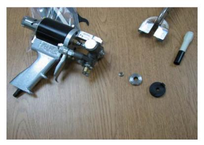
The GX-7 uses a mixing module to properly mix and atomize the A and B components within the gun. The modules are available with various hole diameters based on the application and required output. Please consult NCFI Polyurethanes for recommendations.
